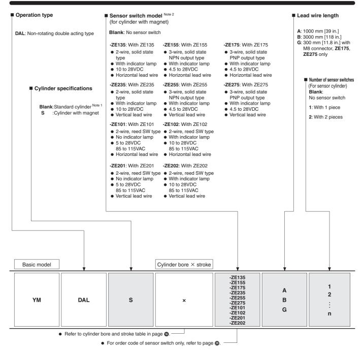
Note 1: The standard cylinder does not have built-in magnet for sensor switch.
