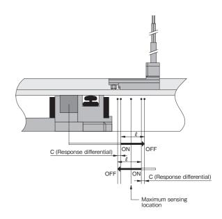
When the sensor switch is mounted at the position specified in the following diagram (values in the table are reference values), the magnet moves to the maximum sensing location position of the sensor switch at the stroke end.
