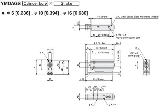
Note: Not available for  $\phi$  6 [0.236] and  $\phi$  10 [0.394] with strokes below 30, and  $\phi$  16 [0.63] with strokes below 20.
