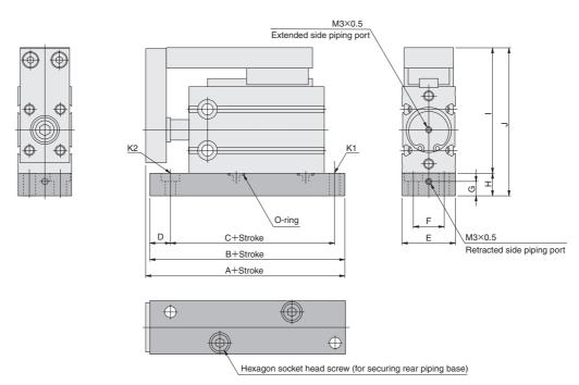
Note: Rear piping base, 2 hexagon socket head screws (for securing rear piping base) and 2 O-rings are included with shipment.
