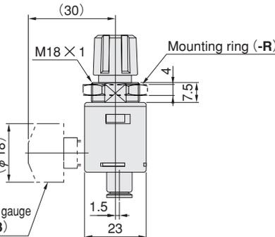
Note: The required mounting hole when the regulator is installed to a panel, etc., is φ 18.5 [0.728in.].
