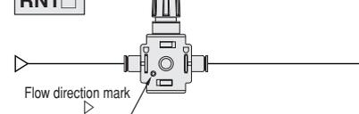
4. When mounting single units of the Compact FR Series, use either the body mounting holes or brackets (optional). Mounting rings (optional) can also be used for panel mounting. The mounting hole for mounting on panels, etc., is  $\phi$  18.5 [0.728in.].
