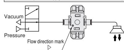
● For side piping regulators and filter regulators, the flow direction mark (▷) is located as shown in the figure below.
