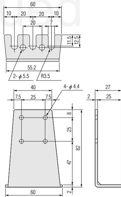
The mounting bracket can be used on the PS2 in either direction.
