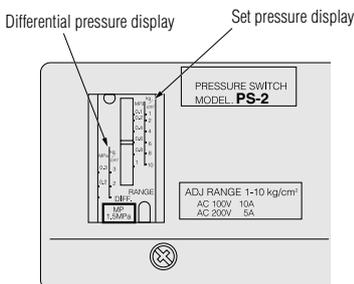
Caution: The number indicated on the dial can be in error for up to  $0.05\text{MPa}$ . For fine adjustment, confirm switch operation by adding compressed air to the set pressure.
