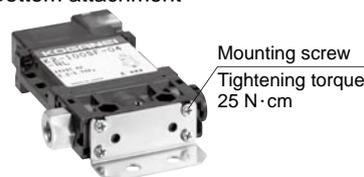
The recommended tightening torque for the valve mounting screws when mounting a valve on the sub-base is shown on the right.
