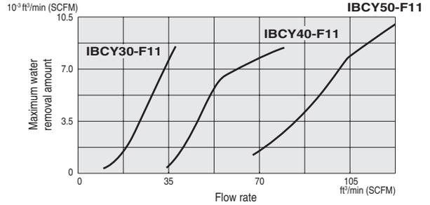
Note: The maximum amount of water removed from a volume of air in a process depends on the conditions of usage (this graph is not a guarantee). Use it as a guideline for your selection.
