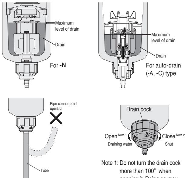
Note: Cut the end of the tube connected to the fitting straight across, and insert completely and securely as shown in the diagram. Also, after installing it, lightly pull it to confirm that it does not come out.
