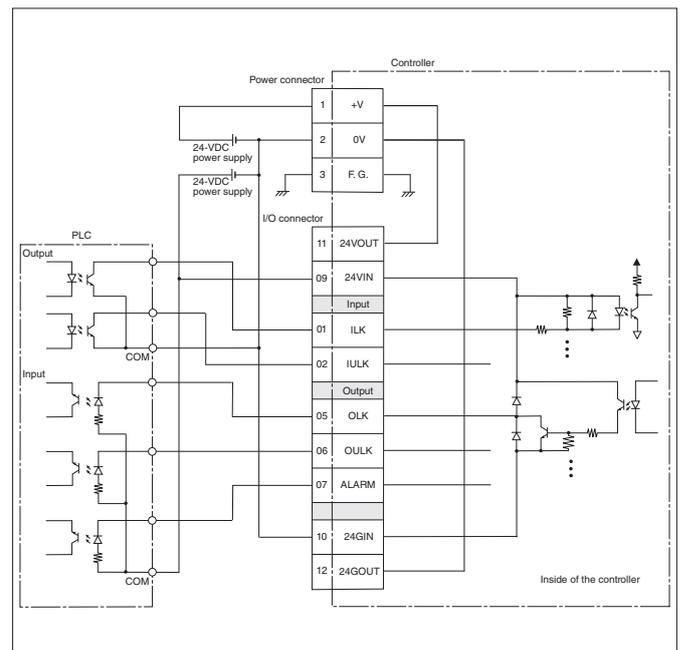
\* Even for just input or output, connect the power supply to 09 and 10.
