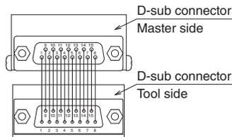
Note 1: The pin numbers for the 15 electric contact pins are connected so they are the same on the master side and the tool side.
