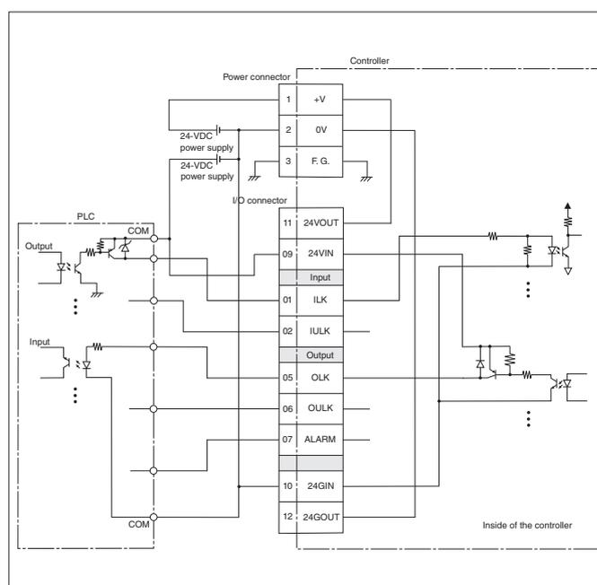
\* Even for just input or output, connect the power supply to 09 and 10.
