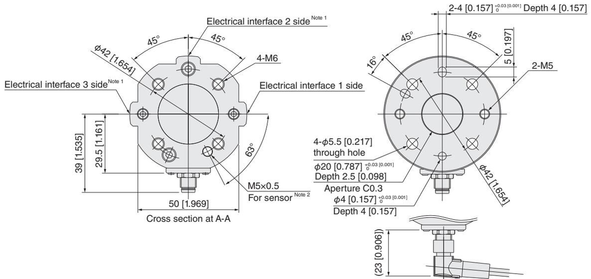
When relay cable is connected (-3L, -5L)
