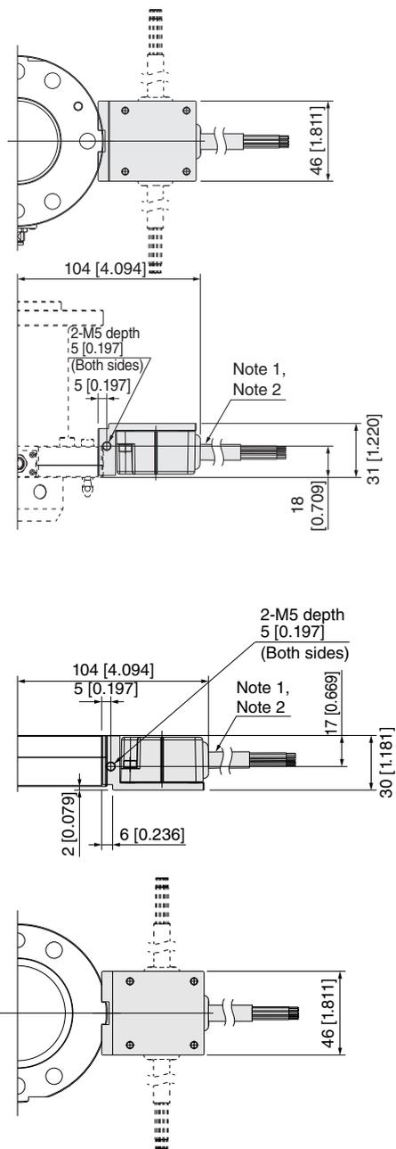
Note 1: For the non-contact terminals (-R), only the adapters are shipped assembled.
