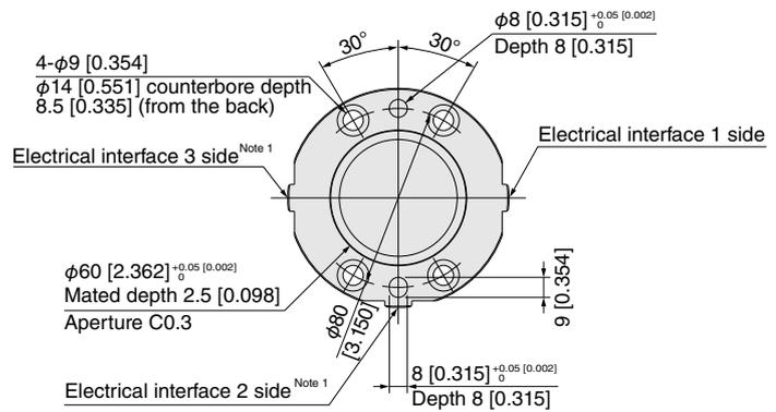
Note 1: For dimensions of the electrical interface 2 side and 3 side, refer to the electrical interface 1 side.
