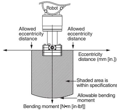
Step ① Select the size model in which the tool load  $W1$  and the eccentricity distance  $L1$  when lifting satisfy the allowable eccentricity distance  $A1$  in graph 1.
