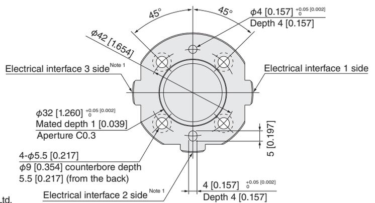
Note 1: For dimensions of the electrical interface 2 side and 3 side, refer to the electrical interface 1 side.
