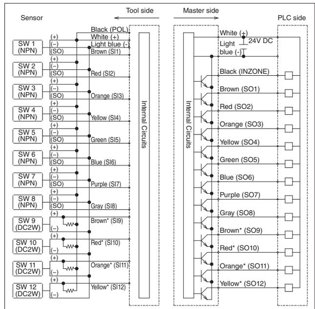
■ SW9 to 12 in the above diagram are examples using DC 2-wire wiring (use wiring for resistance of about 1 to 2 KΩ). DC 3-wire sensors can also be used.
