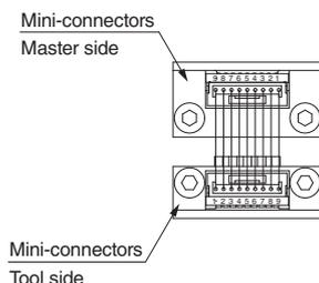
Note 1: The pin numbers for the 9 electric contact pins are connected so that the master side and the tool side are reversed.
