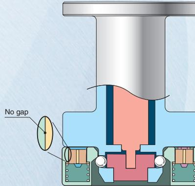
The master side approaches the tool side, and sends a lock signal to the motor.
