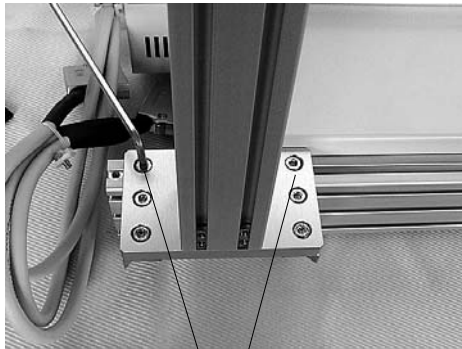
● Vertical stand mounting bolt
