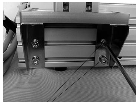
● Vertical stand mounting bolt
