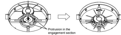
Note1: Turn the discharge needle unit until securely locked. The correct installation of the discharge needle unit on the Main Unit is essential for the optimum operation of the Product.
