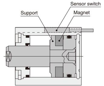
● The diagram is for  $\phi 12 \sim \phi 100$ .
