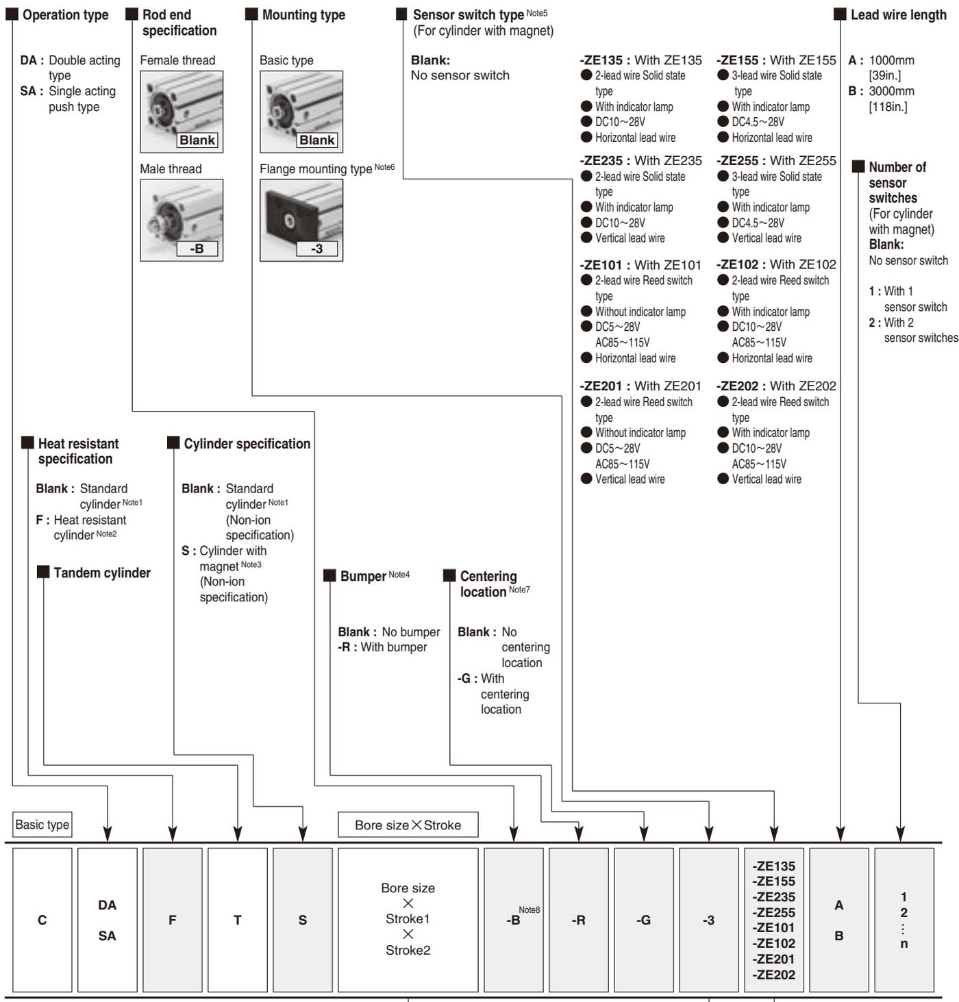
● See table for bore size and stroke. ● Mounting brackets are included at shipping.
