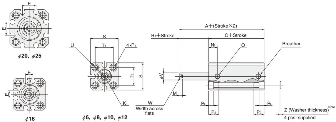
Note: Bore sizes  $\phi 6$ ,  $\phi 8$ , and  $\phi 10$  are not available with washers.
