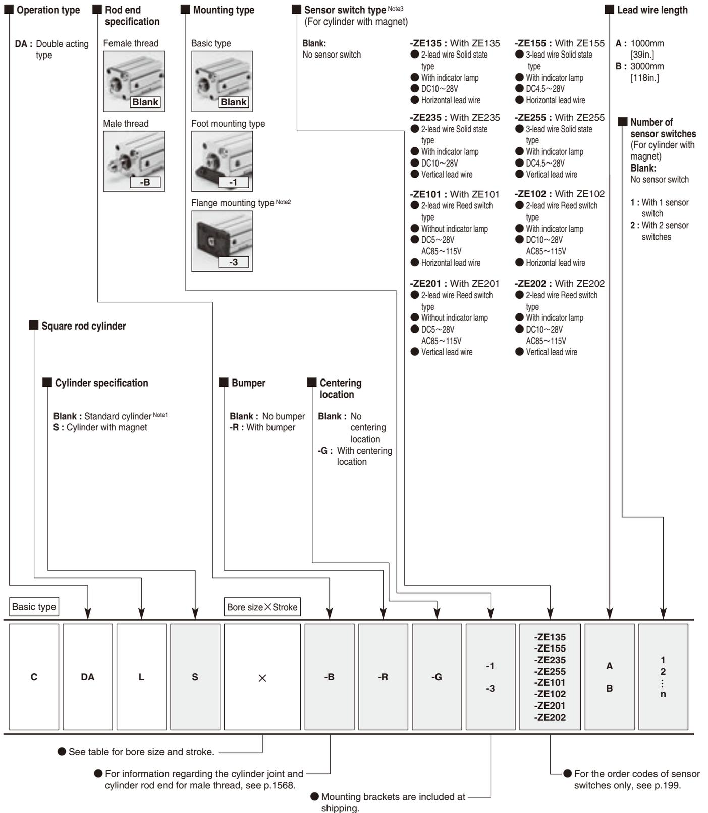
Notes: 1. In the standard cylinder, a magnet for the sensor switch is not built-in.
