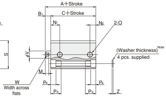
Note: Bore sizes  $\phi 6, \phi 8,$  and  $\phi 10$  are not available with washers.
