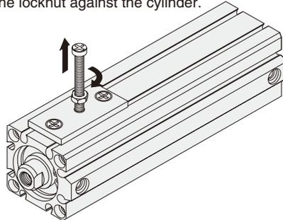
Notes: 1. It is dangerous to release the lock when a load (weight) is present on the piston rod, because it may cause a sudden fall or cause the unintended piston rod's extension (retraction). In this case, always supply air to the connection port opposite the one adjacent to the locking mechanism before releasing the locking mechanism.
