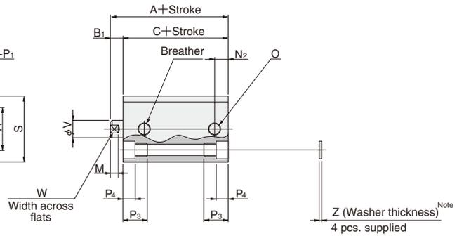
Note: Bore sizes  $\phi 6$ ,  $\phi 8$ , and  $\phi 10$  are not available with washers.
