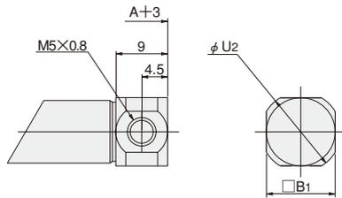
● Lateral piping with mounting thread (-M)
