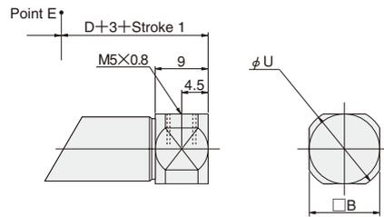
● Lateral piping with mounting thread PBDAT  ×  ×  -M
