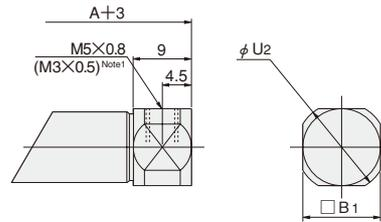
● Lateral piping with mounting thread (-M) Note 2
