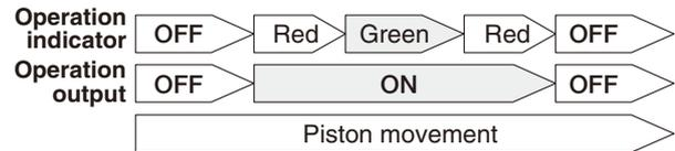
In an unstable range, the red LED lights up, while the green LED lights up when in the setting range.
