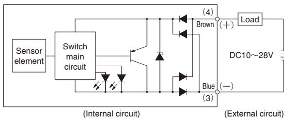
**Caution:** ZD136C is a non-polarity type. Connect either the brown or the blue lead wire to the load.
