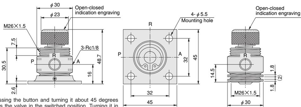
Pressing the button and turning it about 45 degrees locks the valve in the switched position. Turning it in the reverse direction releases the lock, and a spring restores the button to its normal position.
