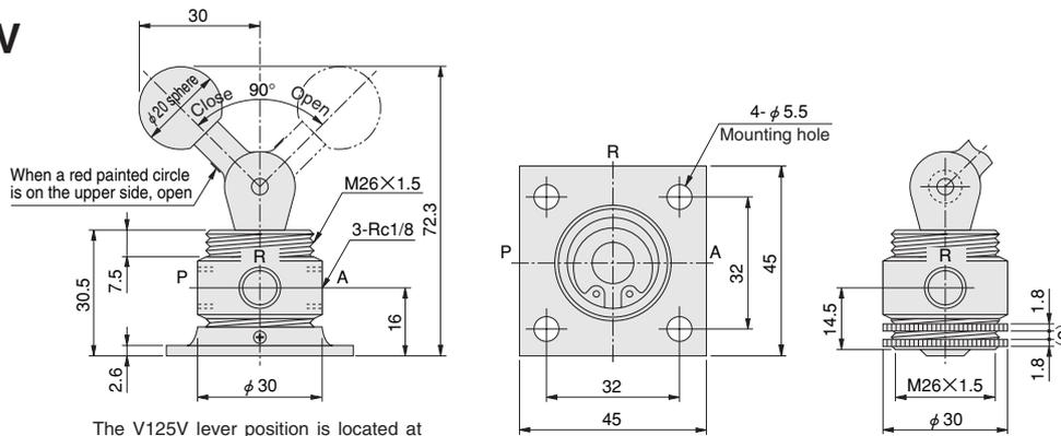
The V125V lever position is located at P side in the normal condition.
