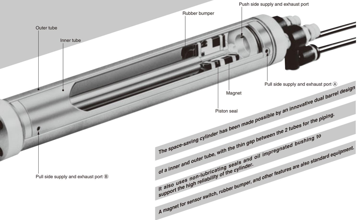
The space-saving cylinder has been made possible by an innovative dual barrel design of a inner and outer tube, with the thin gap between the 2 tubes for the piping.
