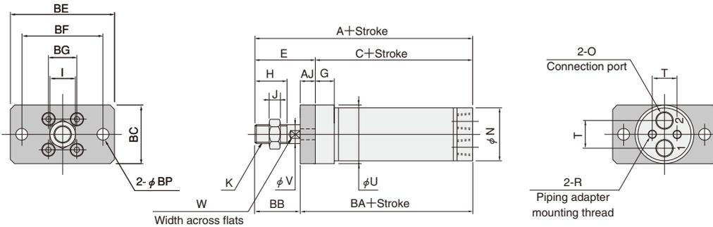
With piping adapter TWDA Bore size × Stroke -HA-L
