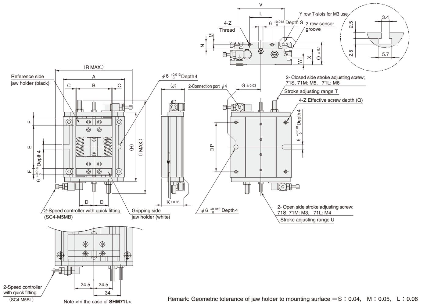
Remark: Geometric tolerance of jaw holder to mounting surface = S : 0.04, M : 0.05, L : 0.06
