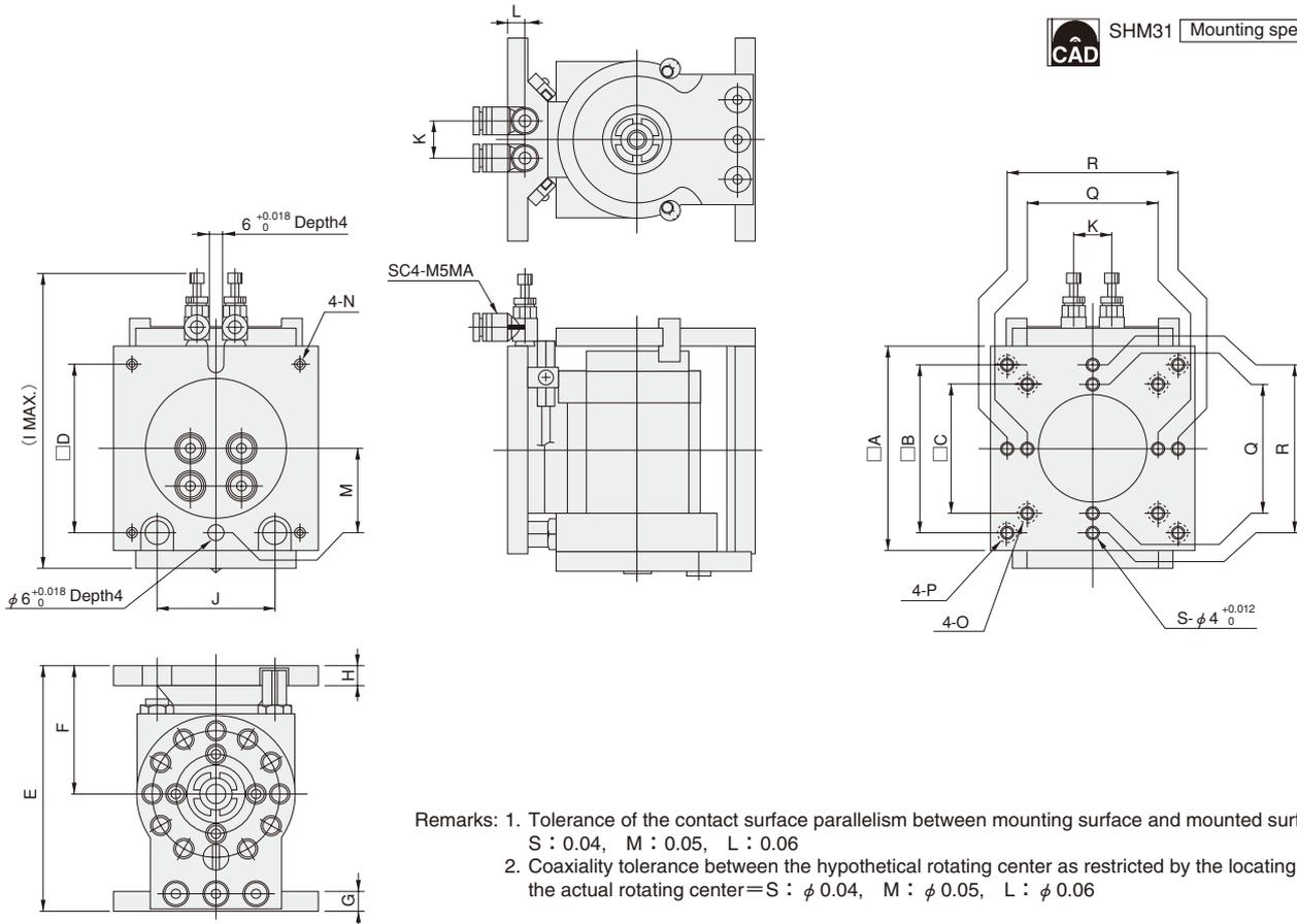
Remarks: 1. Tolerance of the contact surface parallelism between mounting surface and mounted surface = S : 0.04, M : 0.05, L : 0.06
