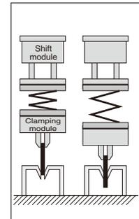
The cylinder inserts the workpiece up to a certain point, after which the spring force provides constant force insertion.
