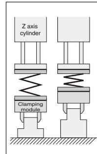
Protects the robot by correcting errors in the height.
