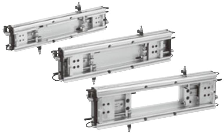
This module plays the role of fingers in the hand (gripper) unit. Because the cylinder is asynchronous, it has superior positioning during clamping. And changing the applied air pressure can make either side serve as the reference jaw. It is particularly suitable for large-sized workpieces.
