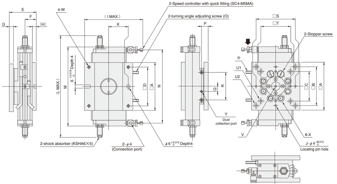
Remarks: 1. Tolerance of the contact surface parallelism between mounting surface and mounted surface = S : 0.04, M : 0.05, L : 0.06
