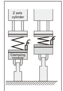
Uses sensor to detect abnormalities in the height, and removes abnormal workpieces only.
