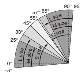
The arrows → show the range of turning angle adjustment by changing the shock absorbers' mounting positions. For adjustment other than that shown above, consult us.
