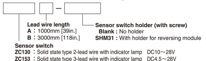
● For details of sensor switches, see p.1544.
