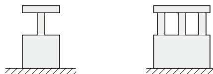
Right angled mounting (2 surfaces and 3 surfaces)
