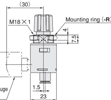
Note: The required mounting hole when the regulator is installed to a panel, etc., is φ 18.5 [0.728in.].
