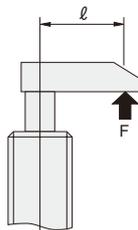
Note : When a Koganei adjusting plate is used for operation, the maximum operating pressure at  $\phi$  16 [0.630in.] is 0.5MPa [73psi.].
