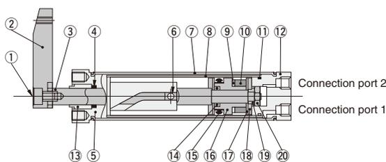
Remark: The positional relationship between the connection ports and the adjusting plate (2) when the piston is retracted is shown in the diagram to the left.
