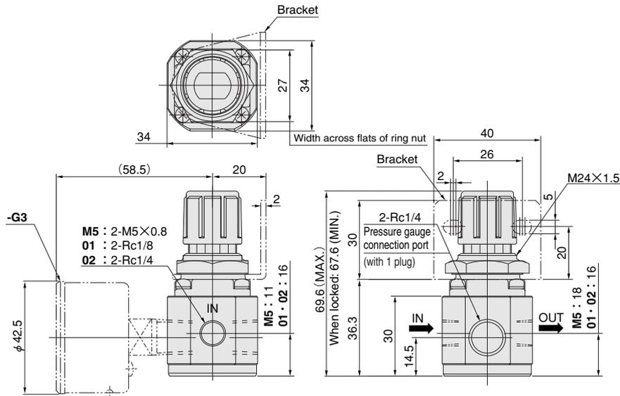
Remark: Mounting holes for the precision stainless regulator on a panel are φ24.5.
