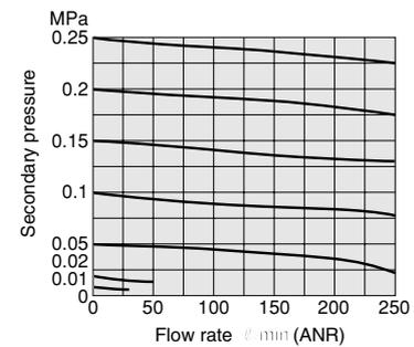
Remark: Graphs show flow rate characteristics when the primary pressure is fixed at 0.7MPa [102psi.].
