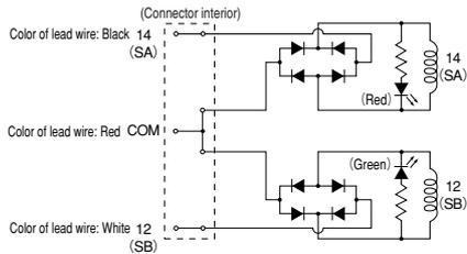
Note: Since there is no polarity, the valve can be used for either +COM or -COM.
