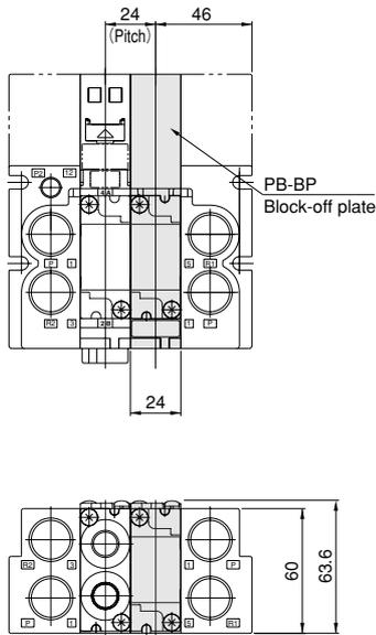
●Individual air supply and exhaust spacer (PB-Z□)
