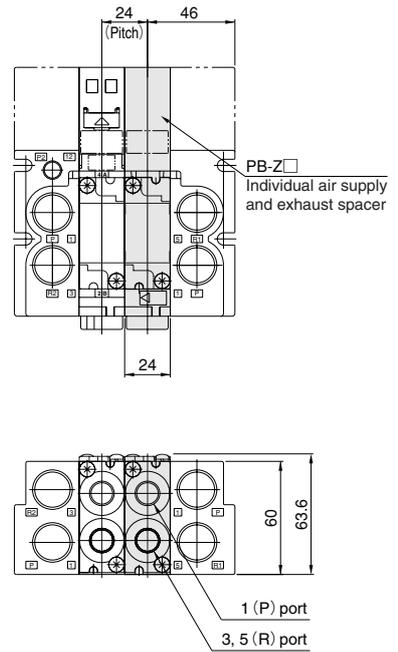
●Safe block Piping specification: Front surface piping (-T□)
