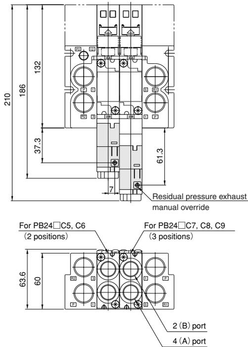
●Safe block Piping specification: Top surface piping (-U□)
