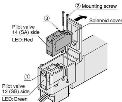
**Caution:** The maximum height of the cover when open is 48mm [1.89in.] from the top surface. Ensure enough space for maintenance, etc.
