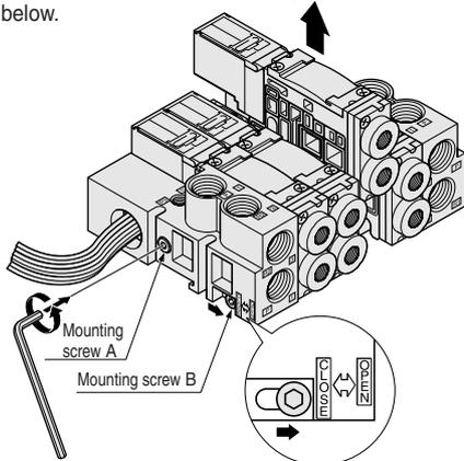
Recommended tightening torque for mounting screws:
