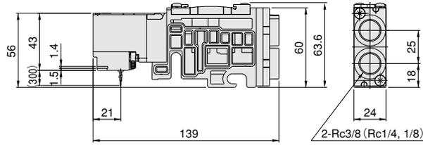
● Piping specification: Top surface piping (-U )
