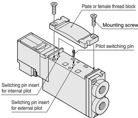
Recommended tightening torque for mounting screws: 137.3N·cm {14.0kgf·cm} [12.2in·lbf]
