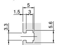
Dimensions of M3 nut groove
