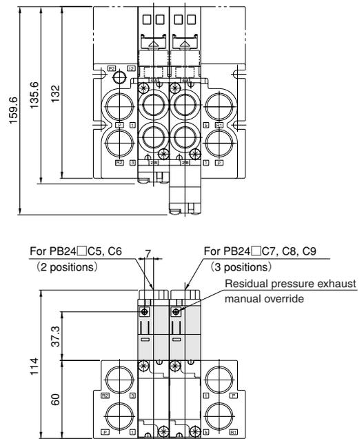
●Dustproof conduit cap: For serial transmission (-FS1)
