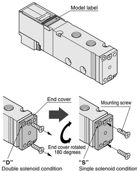
Recommended tightening torque for mounting screws: 88.3N·cm {9.0kgf·cm} [7.8in·lbf]
