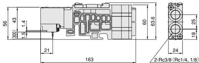
● Piping specification: Top surface piping (-U )
