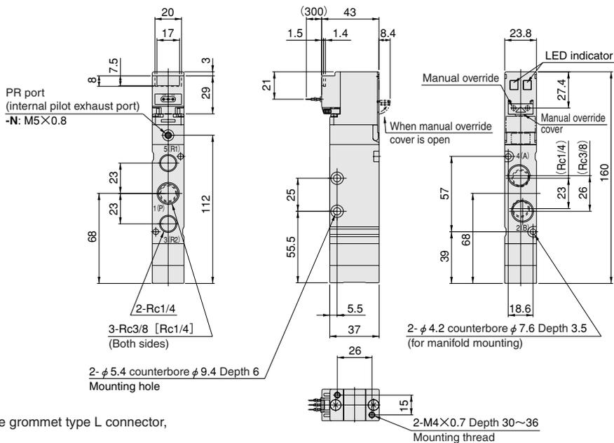
For wiring specifications other than the grommet type L connector, see p.679.
