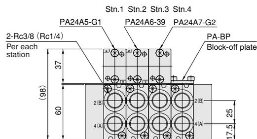
Note: The side piping type and bottom piping type cannot be selected on the same manifold. Select either piping type for the manifold.
