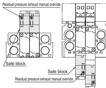
4. To lock the residual pressure exhaust manual override, push the manual override all the way down and rotate it 90 degrees in the clockwise direction. When in the locked state, rotate the manual override 90 degrees in the counter-clockwise direction; a spring returns the manual override to its normal position, and the lock is released. When the manual override is not turned, this type acts just like the non-locking type.
