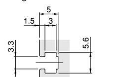
Dimensions of M3 nut groove
