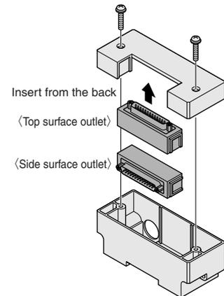
Recommended tightening torque for mounting screws: 58.8N·cm {6.0kgf·cm} [5.2in·lbf]
