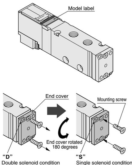
Recommended tightening torque for mounting screws: 88.3N·cm {9.0kgf·cm} [7.8in·lbf]
