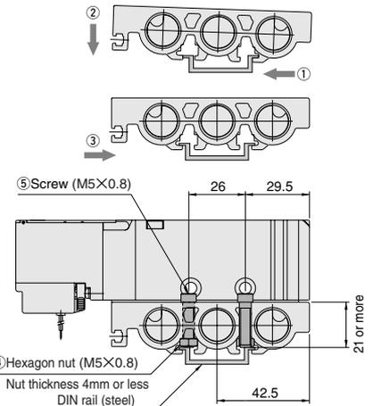
Recommended tightening torque for mounting screws:
