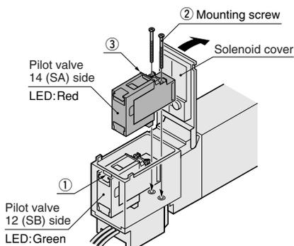
**Caution:** The maximum height of the cover when open is 48mm [1.89in.] from the top surface. Ensure enough space for maintenance, etc.
