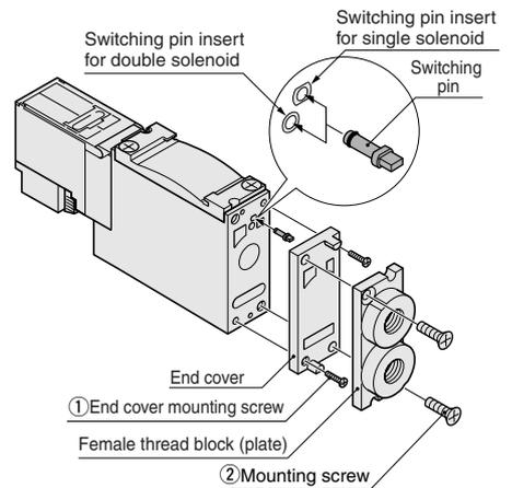
Recommended tightening torques for mounting screws
