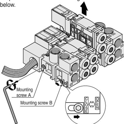
Recommended tightening torque for mounting screws:
