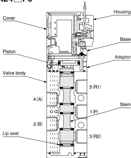
※Schematic diagram shows double solenoid (de-energizing condition after energizing solenoid 12(SB)).
