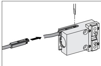
**Caution:** A vertical wire type sensor switch cannot reach the maximum sensing location when it is mounted as shown to the right. Be sure to insert it with the lead wire facing as shown to the left in the illustration.
