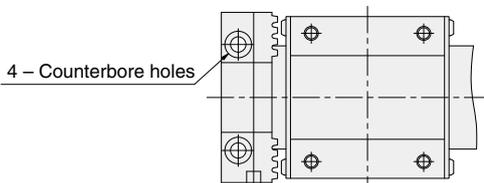
7. Use the M type mount to attach an external guide when using the product. Attaching the guide and slider directly may cause defective operations or malfunctions.
