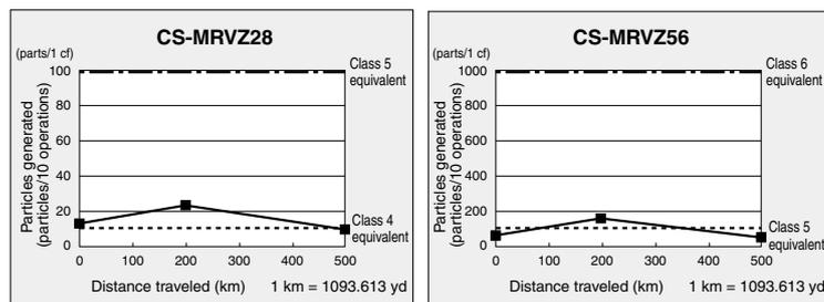
Caution: The particle generation level in the graphs above are based on measured values under conditions established at Koganei and are not guaranteed values.
