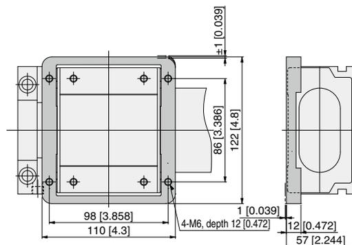
Note: Remove the plate bumper to mount and use the M type mount.
