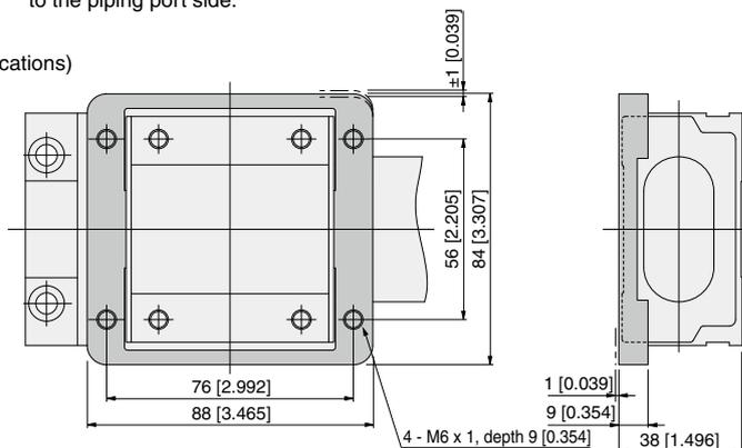
Note: Remove the plate bumper to mount and use the M type mount.
