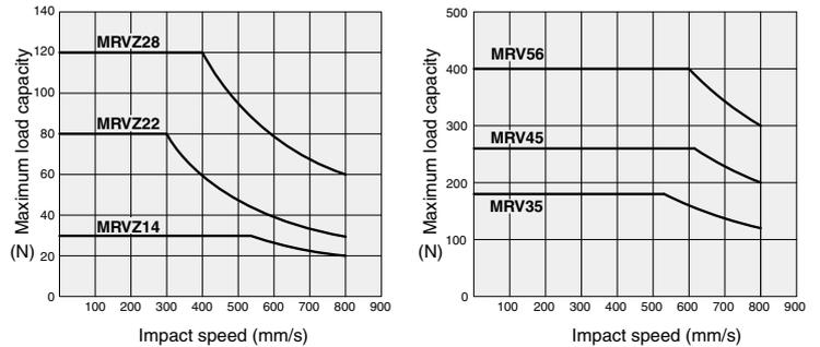
In the graphs, “impact speed” refers to the speed immediately before the slider impacts the rubber bumper or shock absorber.
