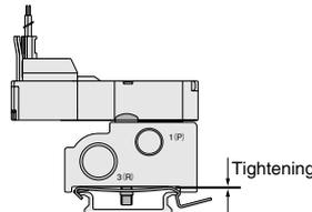
**Caution:** Since the mounting bracket cannot slide along the DIN rail once it is set onto the rail, make sure to set the manifold in the appropriate position beforehand.
