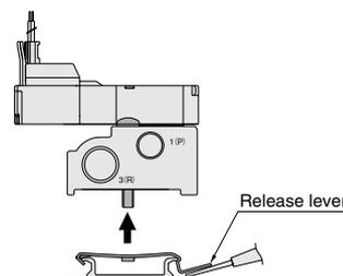
**Cautions:** Spring force from the mounting bracket's plate could cause the bracket to pop out during the removal operation. To ensure safety, proceed with caution during the operation. In addition, always use a flatblade screwdriver, etc. when removing the mounting bracket from the DIN rail. Never use your fingers because of the danger of serious injury due to the potential strong forces.
