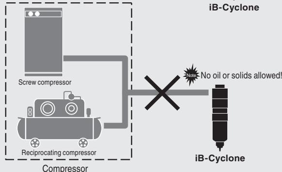
**Note** Perform sufficient countermeasures to remove oil and solids from air when using iB-Cyclone.
