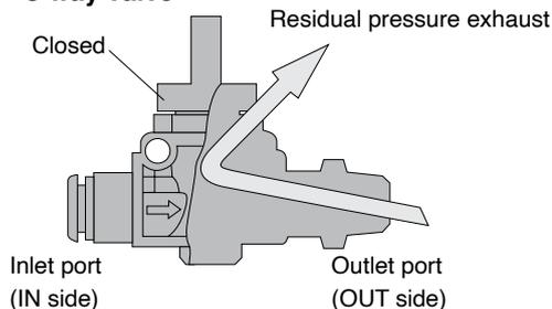
The 3-way valve can exhaust residual pressure (residual pressure remained in installed equipment) left behind in the outlet port side when air has been shut off.
