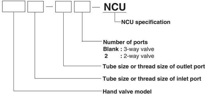
※ For the fitting models, the tube size and thread combinations, see the table below. Columns showing the “←” symbol indicate that standard products can be used as the NCU specification. In these cases, place orders for the standard products.
