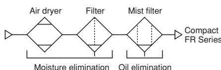
7. The Compact FR Series cannot be disassembled or reassembled. If a filter element reaches the end of its operating life, replace the product with a new unit.
