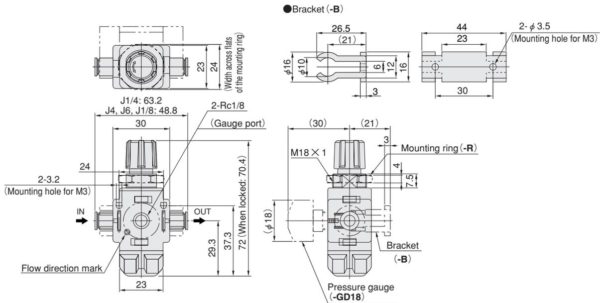
Note: The required mounting hole when the regulator is installed to a panel, etc., is φ 18.5 [0.728in.].
