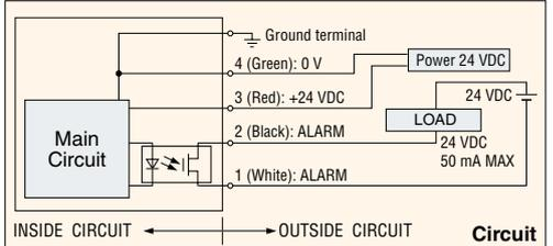
Notes 1: ON/OFF of the power to the Ionizer should be done at the input side (+24 VDC side).
