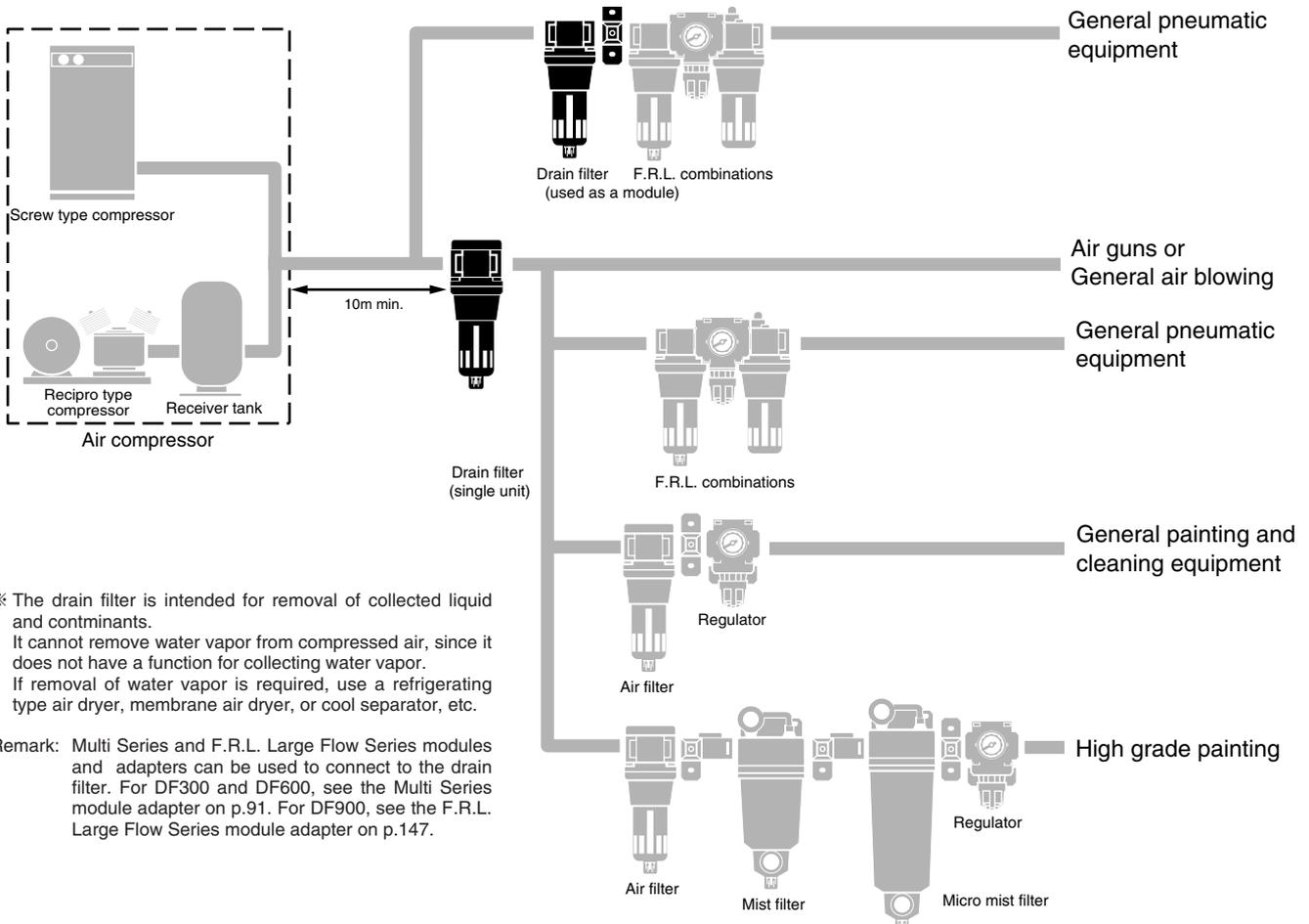
※ The drain filter is intended for removal of collected liquid and contaminants. It cannot remove water vapor from compressed air, since it does not have a function for collecting water vapor. If removal of water vapor is required, use a refrigerating type air dryer, membrane air dryer, or cool separator, etc.
