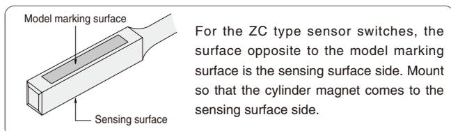
For the ZC type sensor switches, the surface opposite to the model marking surface is the sensing surface side. Mount so that the cylinder magnet comes to the sensing surface side.
