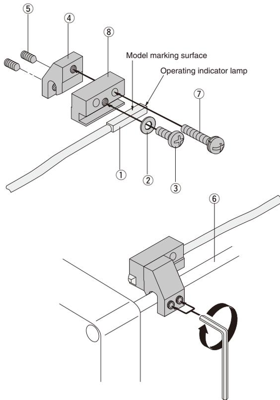
1. ● Align the female thread of sensor holder ④ to the position of the sub-holder ⑧'s thru hole, and use a screw (long) ⑦ to assemble.
