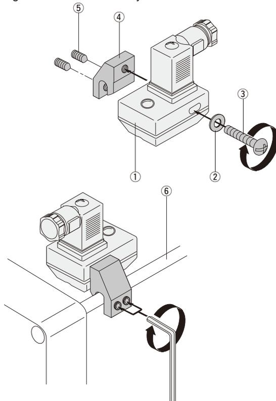
1. ● For the sensor switch ①, align the female thread of sensor holder ④ to any required location of the ①'s thru hole (oval), and assemble.
