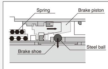
※ Steel balls and a brake shoe are secured in position. Operating the brake piston enables activation or release of the brake.
