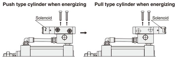
Remove the valve mounting screws, turn the valve 180°, and re-assemble. At this time, confirm that the valve adapter gasket is in the designated position between the valve and the valve adapter.
