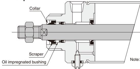
Note: Set the cushion needle tightening torque to 1.0N·m [8.85in·lbf] or less.
