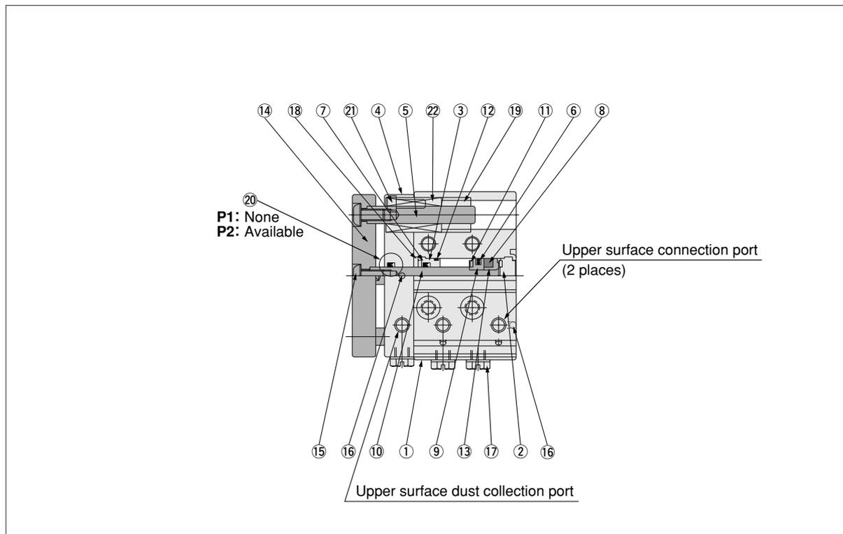
Remark: The number of bearings for 50mm [1.969in.] stroke or shorter is 1 bearing per shaft. At 75mm [2.953in.] stroke or longer, 2 bearings per shaft. The plate, piston rod, and guide rod cannot be disassembled.
