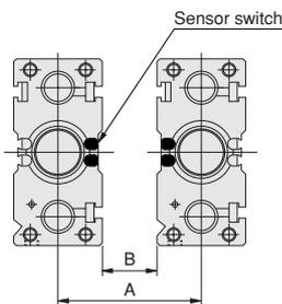
When mounting cylinders in close proximity, install the cylinder so that it exceeds the values in the table below.
