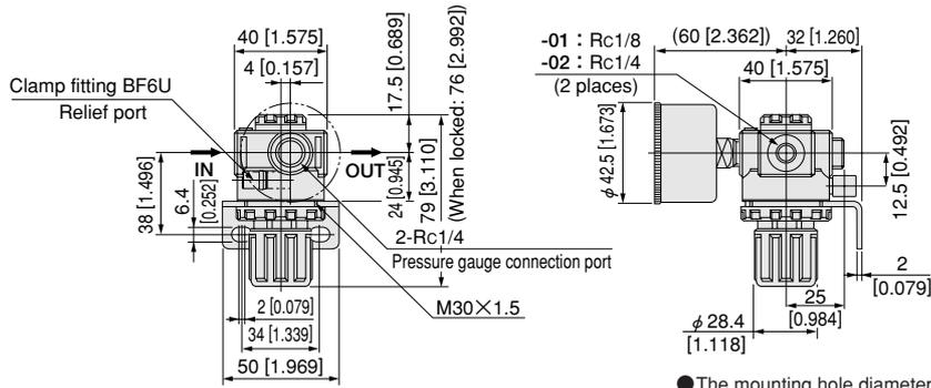
● The mounting hole diameter for mounting the regulator on a panel, etc. should be  $\phi$  30.5 [1.201].
