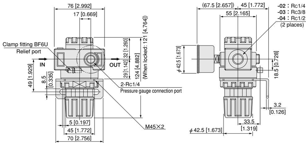
● The mounting hole diameter for mounting the regulator on a panel, etc. should be  $\phi$  45 [1.772].
