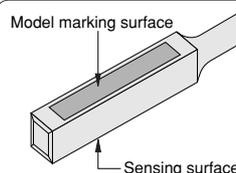
In the ZC type sensor switches, the opposite side from the model marking surface is the sensing surface side. Mount it so that the cylinder magnet comes to the sensing surface side.
