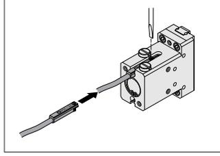
**Caution:** Care must be exercised that a sensor switch cannot be mounted when the body is installed by using thru holes, as shown in the diagram to the right.
