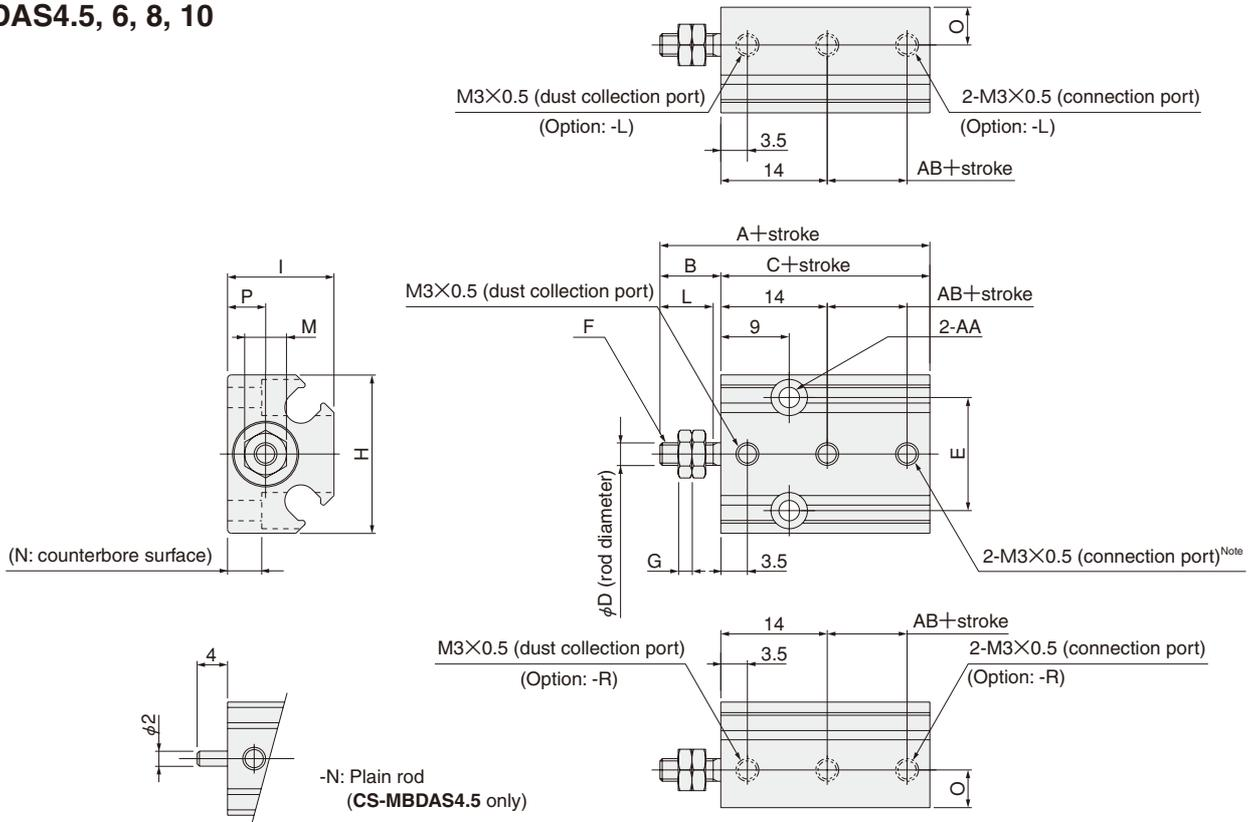
Note: When selecting the optional port location code -R or -L, the standard connection port comes with a plug.
