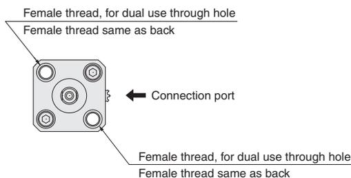
\* The head side (back surface) has dual use female thread/through holes at two locations. The other two locations are female thread only.
