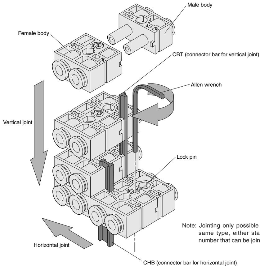
Note: Joining only possible between two units of the same type, either standard or mini. Maximum number that can be jointed vertically is four units.
