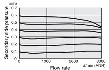
Remark: The graphs show the flow rate characteristics when the primary pressures are constant at 0.7 MPa.
