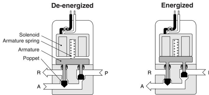
1. When de-energized, air coming through port P is closed by the poppet at P, and air at A goes to port R.
