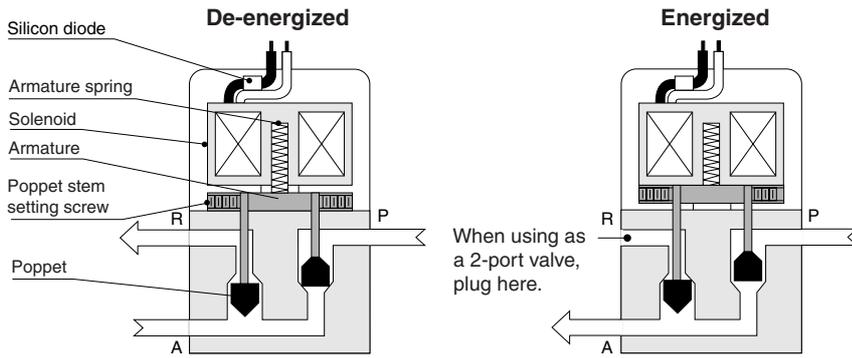
● For the keep solenoid (SE2) type and double solenoid (E2) type, see p.881.
