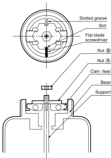
Note: Place the cam under the side with the black mark.
