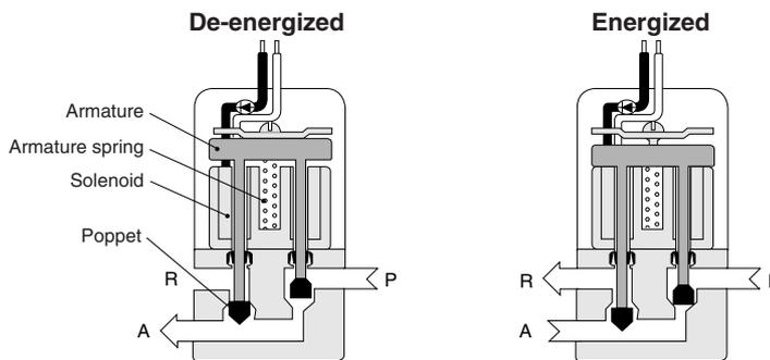
1. When de-energized, the air coming through port P flows to A, but the R side is closed.
