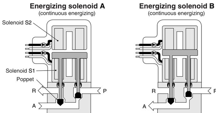
1. When the S1 solenoid is in an energizing condition, the air coming from P is blocked by the poppet at P, and air flows from A to R. This condition is firmly maintained by the air pressure applied to the poppet at P.
