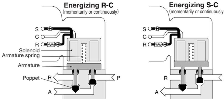
1. When power is supplied to the R-C terminal, the air coming from P is blocked by the poppet at P, and air flows A to R.
