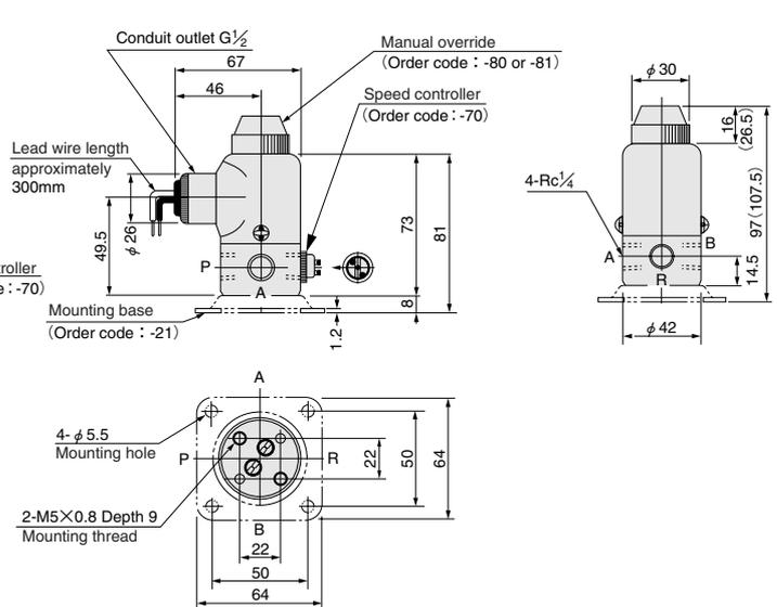
Note: Figures in parentheses ( ) are for the single solenoid with locking type manual override (-81).
