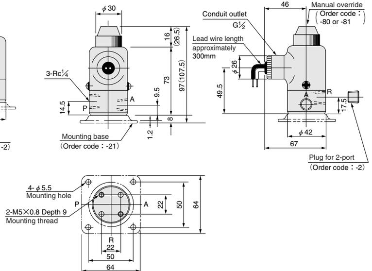
Note: Figures in parentheses ( ) are for the single solenoid with locking type manual override (-81).
