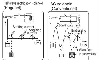
No burning failure will occur even in an abnormal condition.
